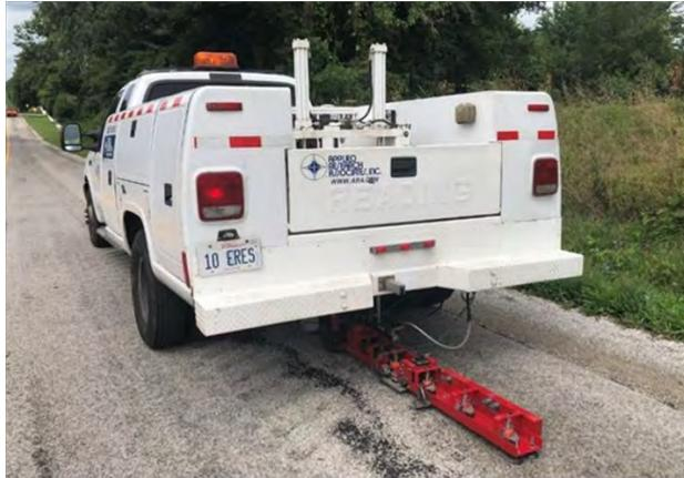
**Figure 3. ARA performs structural evaluation with a truck-mounted FWD.**
